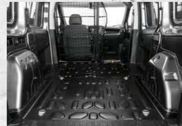
Swivel partition, available for 2 seats configuration only
