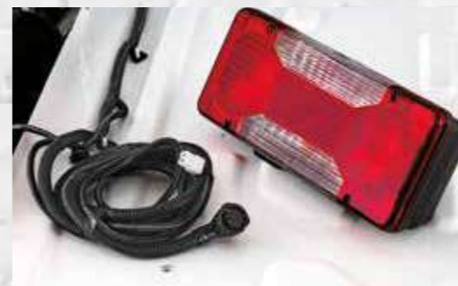
LIGHTING SETUP WITH EXTRA-LONG CABLE AND REAR LIGHT CLUSTER (OPT. 4EA)
