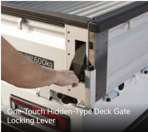
Lightweight Aluminum 3-Way Deck Gates (Anodized Coating)
