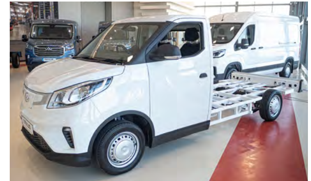
CHASSIS (5144mm Overall Length)
