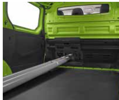
Load through bulkhead flap is magnetised to fix easily and securely in place
