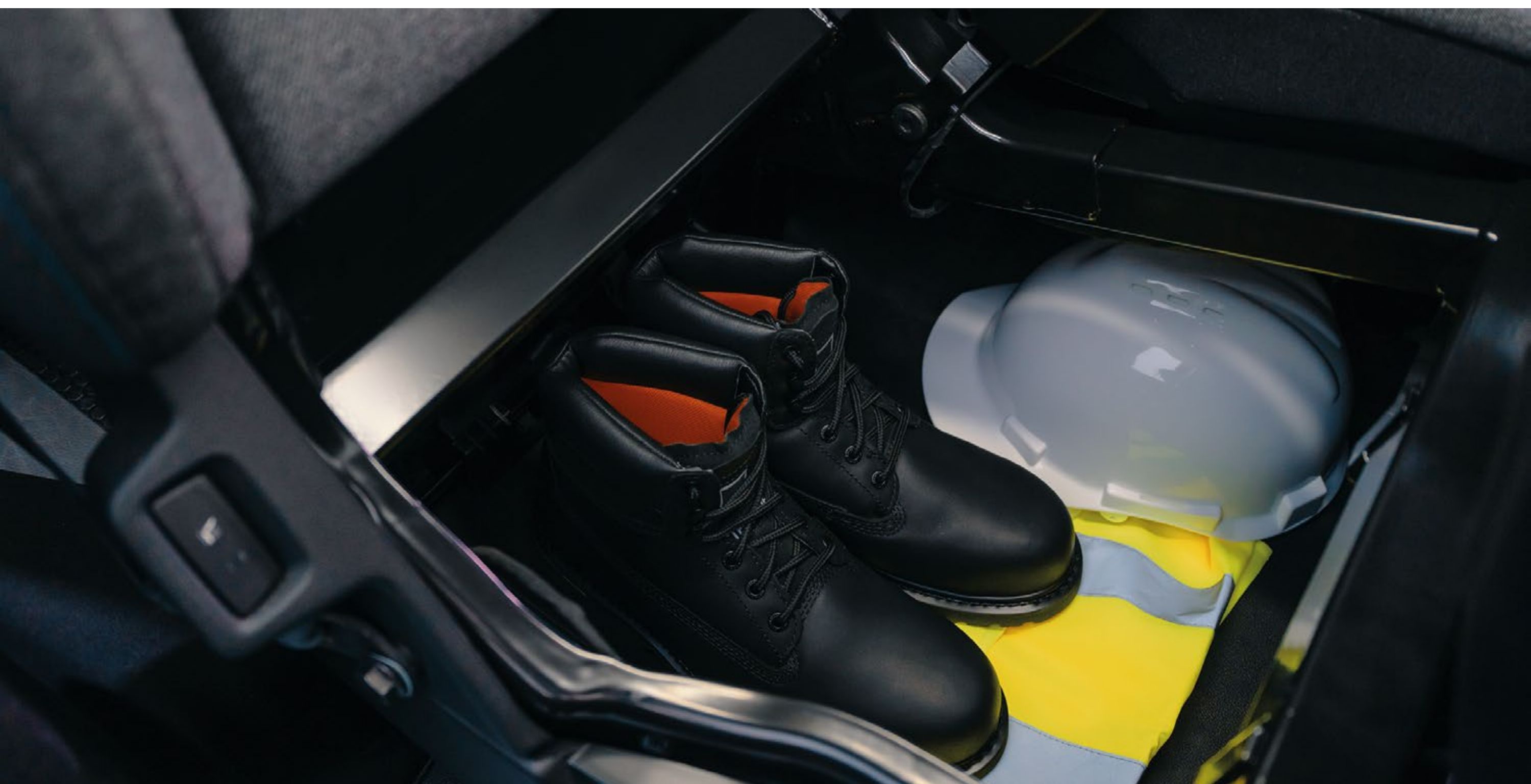
66-litre storage compartment under front passenger seats
