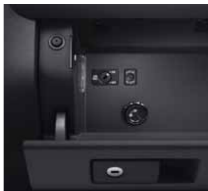
The standard RCD 210 radio has an aux-in socket for your phone or MP3 player
